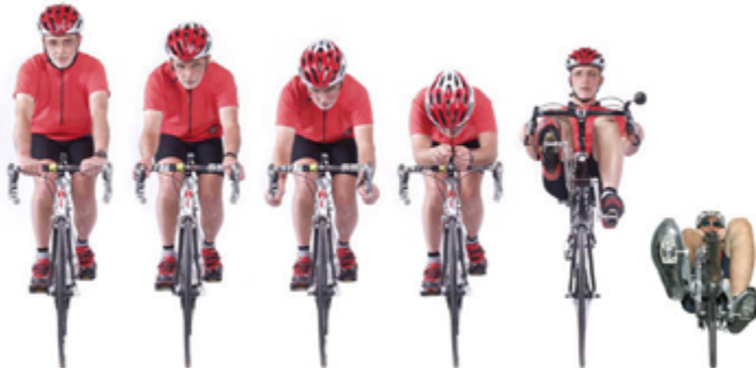
Figure 12. Aerodynamics of a diamond-frame bicycle compared to recumbent models. Image courtesy of Dana Leiberman, Bent-Up Cycles. This image illustrates progressively faster riding positions on a conventional bike and two comparative recumbent positions.
