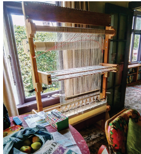
Figure 12. Loom with roller and two shafts containing Texsolv heddles. The shafts were manually operated and held open by a piece of curved wood.
