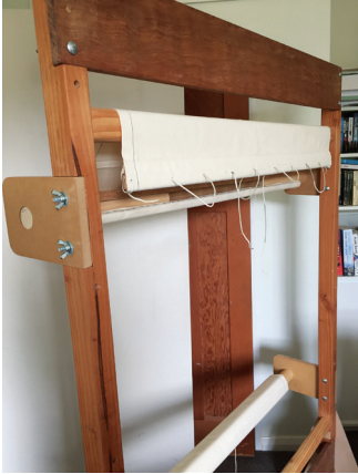
Figure 4. The addition of rollers to the rack loom, using recycled loom parts.
