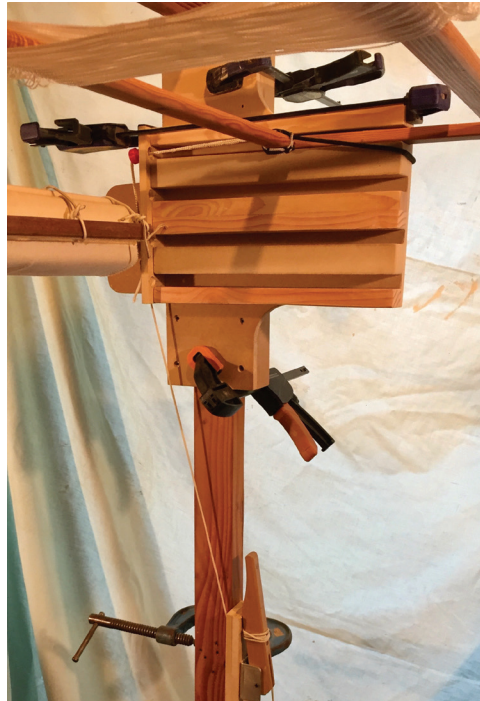
Figure 16. Horizontal castle, demonstrating using the lever with bungee cord.
