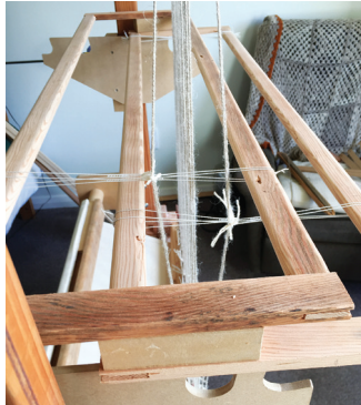
Figure 8. Shafts moving in two directions to create shed.
