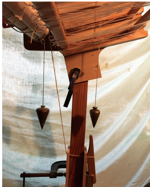
Figure 17. Angled castle, showing the use of plumb-bobs to align the heddles and setup the lead lines.
