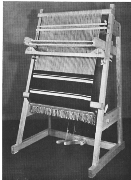
PLATE 3. DRYAD FOOT POWER RUG LOOM.
