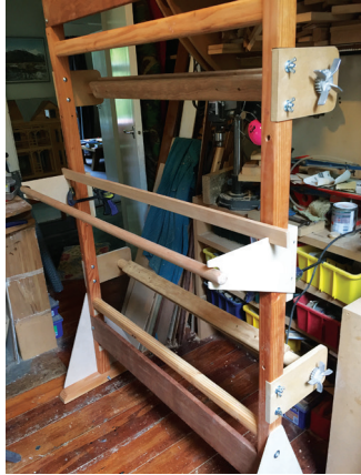
Figure 5. The use of a stick and pole to create a shed.
