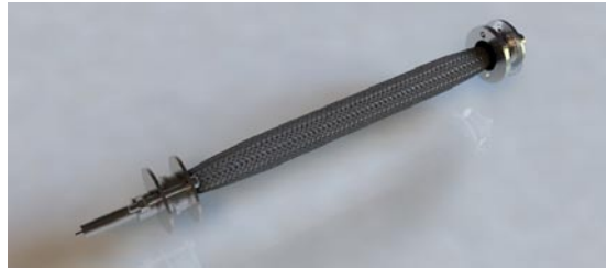
Figure 8: Pneumatic muscle 'deactivated'.
