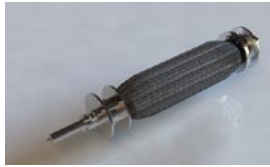
Figure 7: Pneumatic muscle 'activated'.
